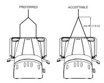
Use a double chain or cable setup that distributes the load equally to both hitches (see either example in Recovery Rigging Options illustration):
