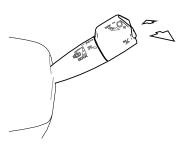
When in the Manual mode, the transmission gears can be manually selected by pushing or pulling on the lever. Pushing the lever forward will down shift. Pushing and holding the lever forward will engage the LOW gear range. Pulling the lever towards the driver will upshift the transmission.
