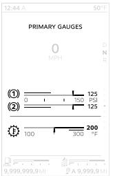
A gauge view presents the standard and optional virtual gauges monitoring your truck systems. Two single or two compound gauges can be shown per view. Gauges not shown in the first gauge view are shown in additional gauge views until all monitored systems are represented:
