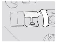
Press the lever down to engage the Trailer Hand Brake. Push the lever back up to release the Trailer Hand Brake.
