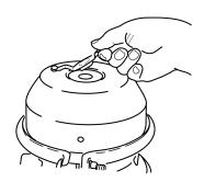
Remove the release stud assembly from the side pocket, and remove the release nut and washer from the release stud.
