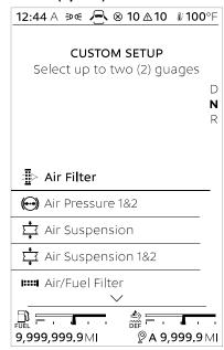
Vehicles with this option provide a view which can contain up to four operatorselected gauges. If the custom view has not been configured, scrolling to the custom view allows the operator to enter the custom view setup (See Custom Setup).<sup>7</sup> The custom view can also be changed in the menu.
