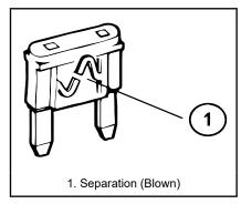
3. If it is blown, replace it with a fuse of the same rating. If a fuse of the same rating is not available, a fuse of a lower rating may be temporarily substituted. You can also use a fuse from a circuit you can do temporarily without (for example an accessory circuit or radio).
