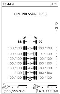
The Tire Pressure Monitoring System (TPMS) is an optional feature combining tire data with the chassis axle layout, displayed graphically. The TPMS can be
