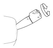
The transmission mode is selected by rotating the lever outer knob. There is a position for Drive (**D**), Neutral (**N**), and Reverse (**R**) and for some vehicles Park (**P**).
