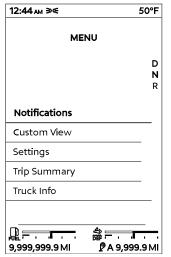
The menu allows the operator to view active warnings, truck performance, activate and customize vehicle features, and access trip information. The menu can only be accessed when the parking brake is set.<sup>8</sup> Use the **Scroll** to choose the menu
