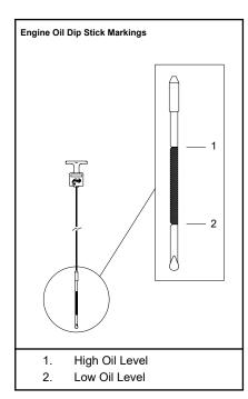
7. Reinstall the dipstick and twist to lock it in place.
