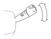
Moving the shifter down (clockwise) will engage the engine brake, with each downward position providing more engine braking. The bottom-most position (Position 4) is a momentary position and activates MAX mode.
