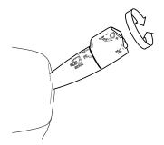
Transmission mode is selected by rotating the lever outer knob. There is a position for Drive (**D**), Neutral (**N**), and Reverse (**R**). The Digital Display will indicate the corresponding mode. See *Drive*, *Neutral*, and *Reverse Indicator*.
