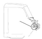
Locate the filter cover labeled "OPEN" with an arrow pointing towards the rear of the vehicle. Slide the filter cover towards the rear of the vehicle, until you are able to remove the cover.
