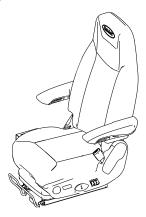
The seats in this vehicle are equipped with a switch that locks out the fore-aft isolator function in the seat. When locked, the seat will not move back and forth. It will be rigidly fixed and only allowed to move up and down with the vehicle's movements. This vehicle may be equipped with a swivel function on the passenger seat. This function allows the passenger seat to rotate and face towards the inside of the cab.
