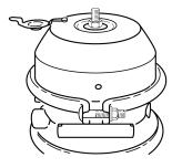
6. With a wrench, turn the release stud assembly nut until the compression spring is 90-95 percent caged. While doing this, ensure the push rod (adapter push rod or service push rod) is retracting. DO NOT over-torque the release stud assembly. (S-Camtype maximum: 50 lb-ft (68 N·m), Wedge-type maximum: 30 lb-ft (41 N·m)). The spring brake is now mechanically released.
